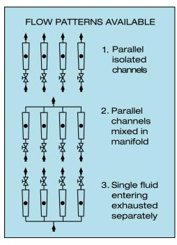
When meters with valves are ordered the valve cartridges are installed at the inlet.
