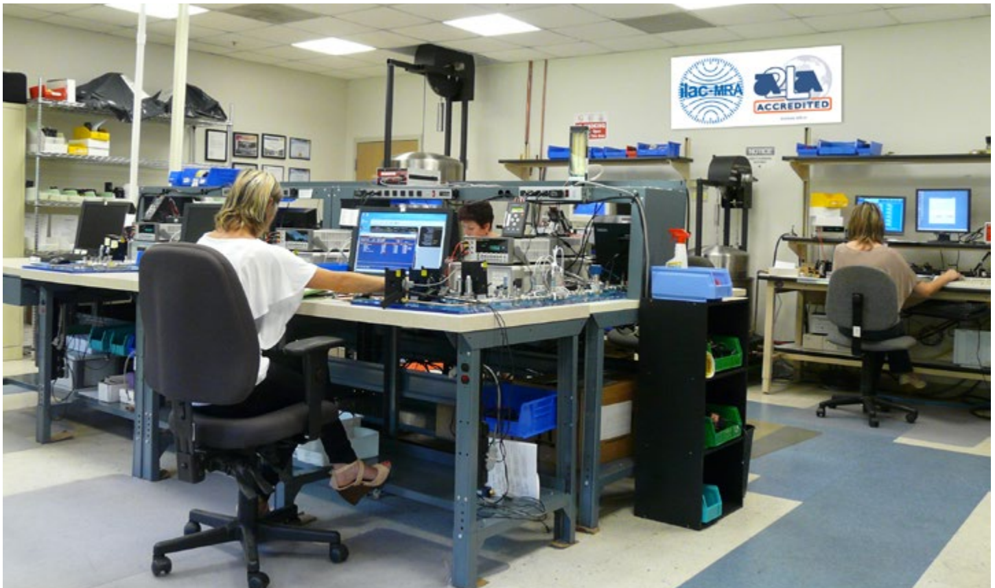
Technicians calibrating Flow Controllers using Bell Provers and Molbox/Molblocs technology.
