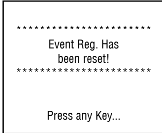
Figure 47: Alarm Event Register Reset Confirmation
