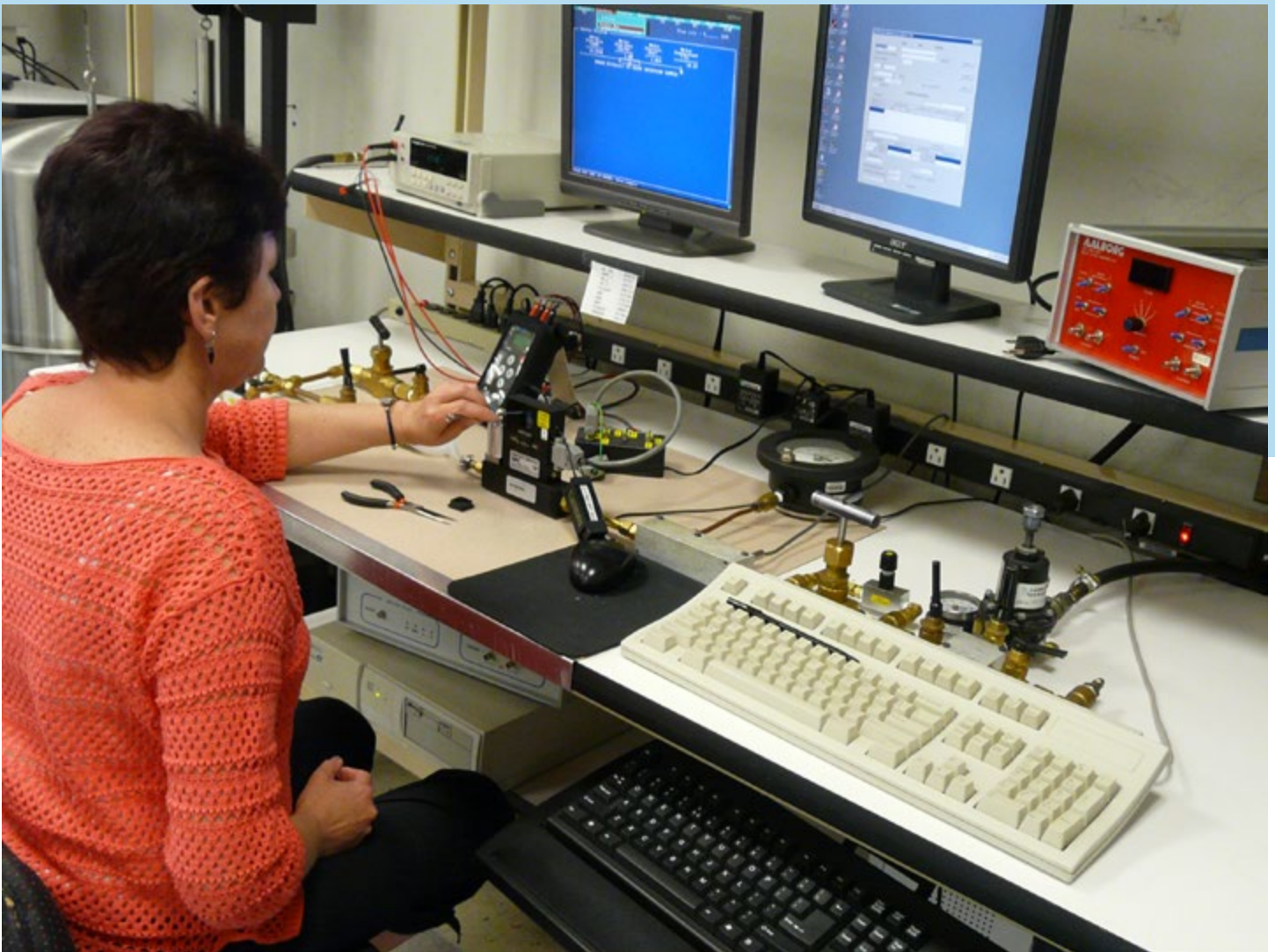
Terminal shown for low-flow Flow Controller calibration supported by Aalborg SDPROC software.
