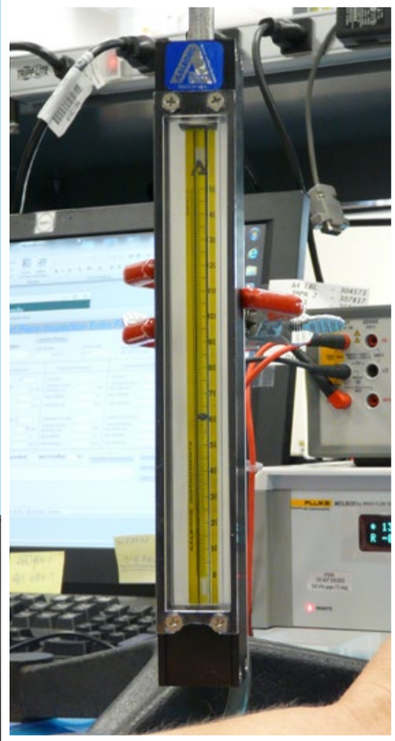
Customer's Rotameter returned for re-calibration performed in Aalborg's laboratory.
