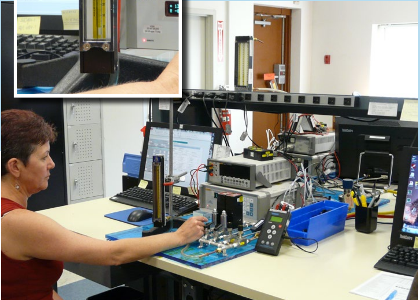
Customer's Rotameter returned for re-calibration performed in Aalborg's laboratory.
