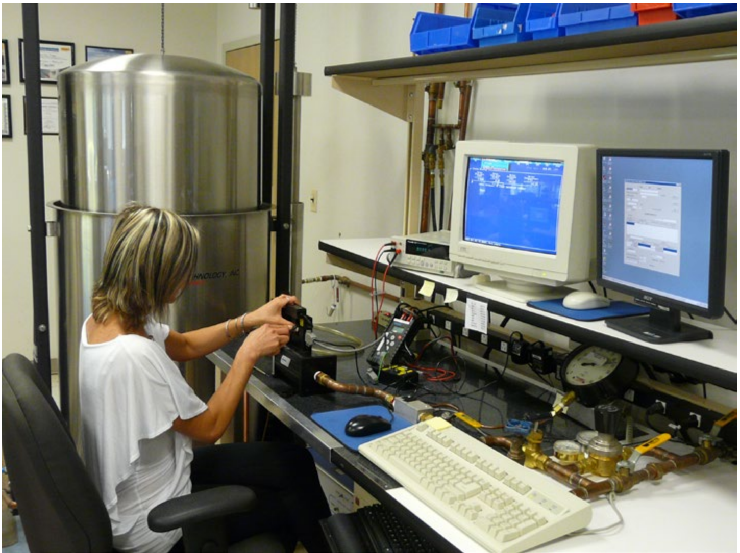
Bell prover used by technician in calibrating high flow capacity Flow Meter.
