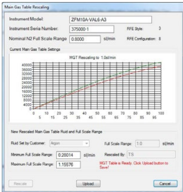
Figure 9.3 Main Gas Table Rescaling using "ZFM Configuration Utility" software: Uploading new MGT to the EEPROM.
